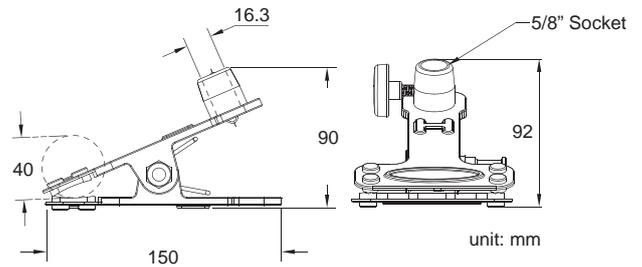
A handy multi-purpose steel clamp which features three attachment methods: a spring-tension with rubber feet protection clamp which has a clamping range of 5-40mm, a 5/8" female socket and a 5/8" stud so it can mount into a lighting stand, Convi Clamp, Super Viser or Grip Head to hold reflectors, gels, foam cores or a flash securely in the studio and on location.
