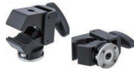
Aluminum alloy clamp equipped with a M6 internal female thread designed for mounting Arri standard rosette-style accessories and it allows 360 degree rotation. The compact super claw clamp offers a great mounting solution which fit tube sizes from 13mm to 35mm or a flat object from 5 to 20 mm.
