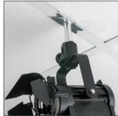
The Kupo Ceiling Frame Mount with Male Spigot Adapter is designed to attach to the metal frame which supports your ceiling tiles. This ceiling clip bracket mount has a 5/8" male stud that accepts lighting fixtures or any compatible 5/8" receiver accessory. Additional 1/4"-20 female thread on the top of baby pin also provides a great mounting solution for a Video/ Audio transmitter.
