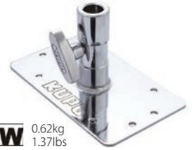
With the same plate size 3.5 x 6" (9 x 15cm) and function as baby wall plate, but welded with a 5/8" baby receiver. Great tool to mount a lighting fixture or grip accessory to a wall. Mount to a baby stand directly or take off the knob for access in to a junior receiver or use as a platform for monitor, speaker or lighting fixtures.
