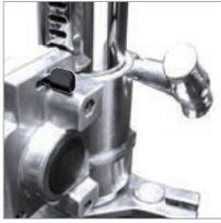
Large size T-handle on each riser is ergonomically design for maximum torque.
