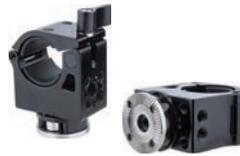
The lightweight aluminum tube mounting coupler designed for DJI Ronin, Freefly Movipro or any Gimbal support system comes with dia. 25-30mm tube. Features a M6 internal female thread designed for mounting Arri standard rosette-style accessories and it allows 360 degree rotation.
