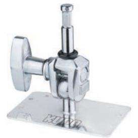
The square plate attached to the ball joint pivots from -45° to 90° while the collar rotates 360° incorporating another 5/8" pin. Plate size: 3.5 x 6" (9 x 15cm)
