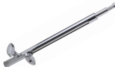
These double riser sections are identical to the ones that come with the Master C-Stands with Turtle Base. C-Stands get their sizing from the length of their riser sections. The 30" double riser for instance, has two (double riser) telescoping risers and one main section for a total of 90". Add the height of the base and you arrive at your maximum height, 2 risers, 3 sections (Dia.: 35mm, 30mm, 25mm)
