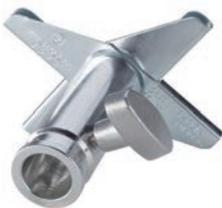
The Kupo Ceiling Clip Female Bracket is an adapter designed to clip on the metal part that supports your ceiling tiles and presses its other side to secure in place. This ceiling clip bracket mount has a 5/8" receiver with metal fastener that accepts lighting fixtures or any compatible 5/8" stud accessory.
