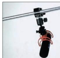
Microphone with Mini Ball Head and Cold Shoe mount on the Gobo arm.
