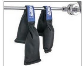
Kupo Shot Bags are made of 1,000 denier black cordex textured Nylon with a water resistant polyurethane coating on the inside. 2mm steel balls are encapsulated in the poly inner bag and sealed up with the bag which makes it dense weight and it never leaks. The two wing design allows it to drape perfectly over light stand legs.
