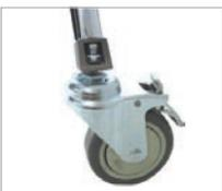
Casters are optional for easily moving the stand. The stand foot is rugged zinc-casting. Dia.: 100mm with brake and M10 attachment. There are three in a set. (KC-100)
