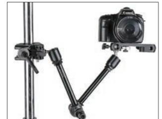
This camera bracket is designed for the Max Arm. Constructed with aluminum die-casting which makes it very lightweight and durable. In addition to a standard 1/4"-20 inch thread mount for a small camera, it also comes with a 1/4" to 3/8" adaptor to accept different sizes of thread mounts. There are four 3/8" female sockets available on the bracket that can connect two max arms from each side giving it the most stability. The 7mm female socket is also built for an umbrella reflector.
