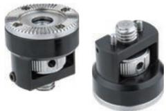
Made by precisely machined stainless steel and aluminum, this Kupo Arri Rosette (60 tooth with 31.8mm in diameter) mount is designed for being attached to cage, rosette handle and other any ARRI standard rosette fitting. The M6 internal female thread designed for mounting Arri standard rosette-style accessories and it allows 360 degree rotation.
